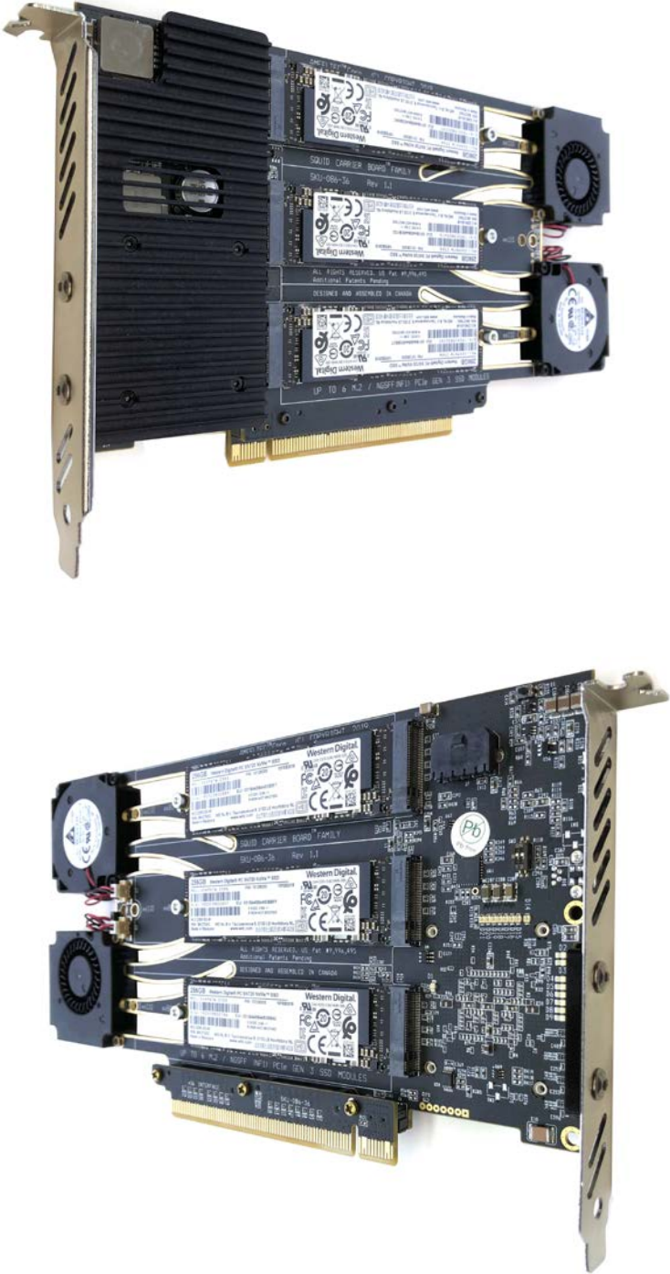
Figure 1: PCIe Gen 3 Carrier Board with six M.2 SSD modules on the top and bottom surface
