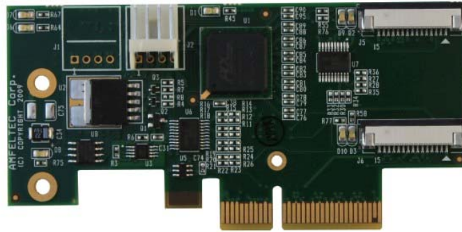
Figure 2: x4 PCI Express Host card (top view)
