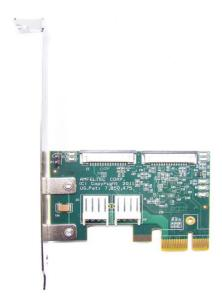
Figure 2: x1 PCI Express Host board (top view)
