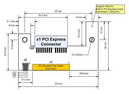
Figure 9: x1 PCI Express adapter board layout
