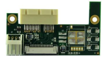
Figure 4: x1 PCI Express adapter board (powered from Host card 12V, 3.3V)
