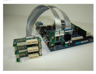
Figure 10: x1 PCI Express adapter boards in combination
