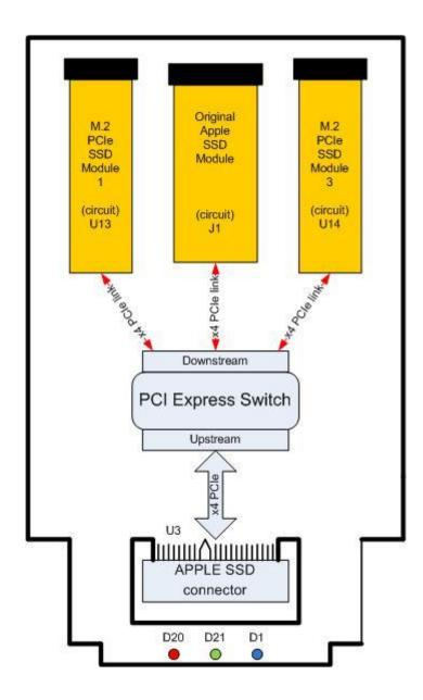
Figure 4: SSD modules to Carrier Board connection diagram.
