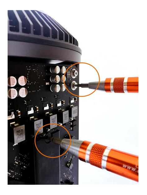
6) Use the screwdriver with "Slotted" bit to *carefully* insert the power standoffs (item #3), as shown.
