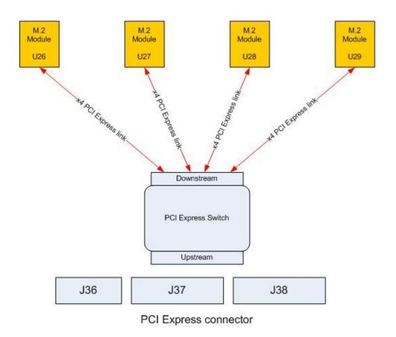
Figure 4: Carrier board PCI Express connection.
