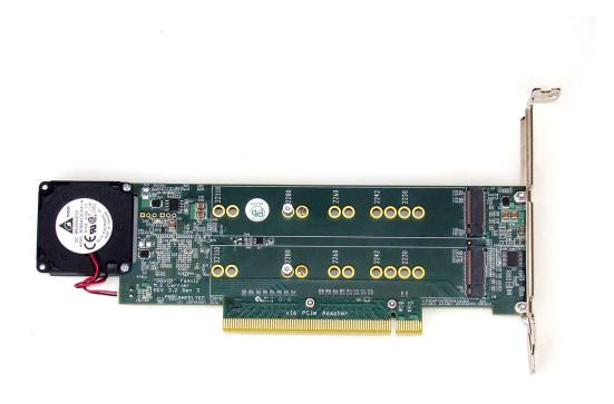
Figure 3: PCI Express Gen 3 Carrier Board for 4 M.2 SSD modules (bottom).
