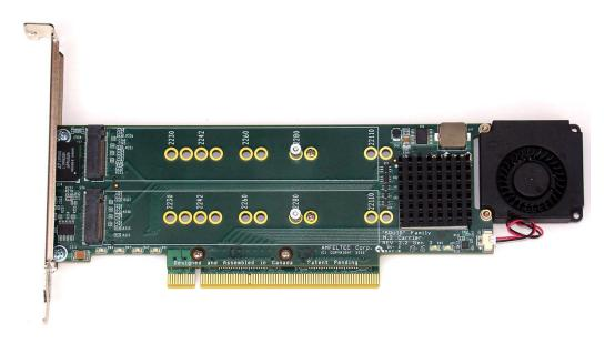
Figure 2: PCI Express Gen 3 Carrier Board for 4 M.2 SSD modules (top).
