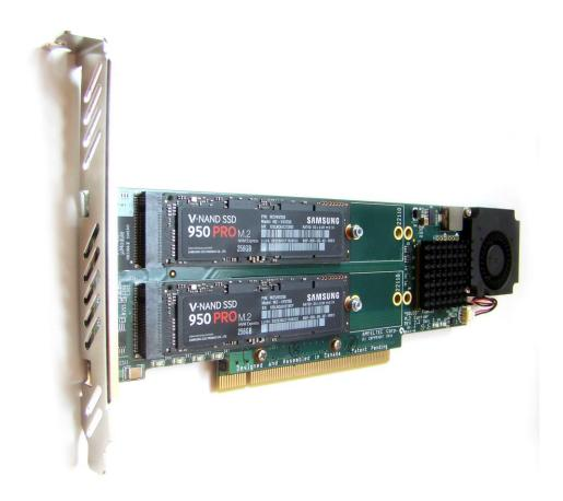
Figure 1: PCI Express Gen 3 Carrier Board for 4 M.2 SSD modules
