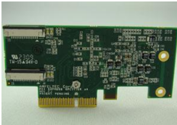
Figure 2: x4 PCI Express Host board (back side)
