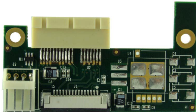
Figure 3: x1 PCI Express adapter board (powered from host card 12V, 3.3V)
