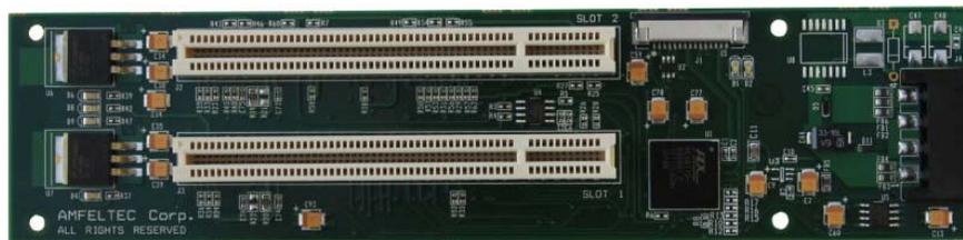
Figure 3: PCI Bus Flex Adapter
