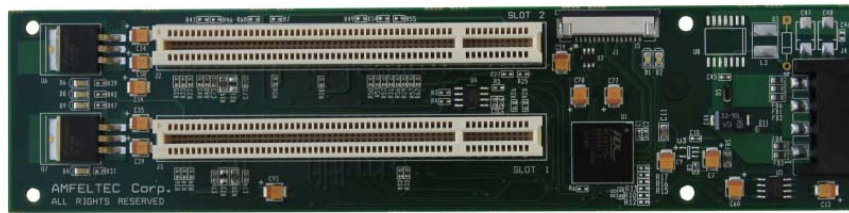
Figure 3: PCI Bus Flex Adapter board
