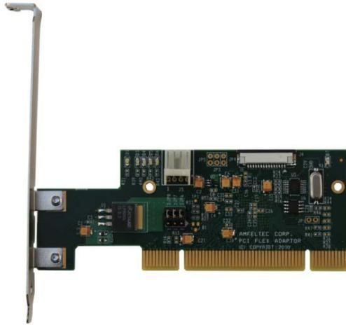
Figure 2: 32-bit PCI Host Card
