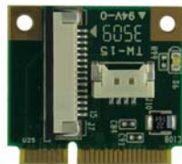
Figure 4: MiniPCI Express (half) Host card
