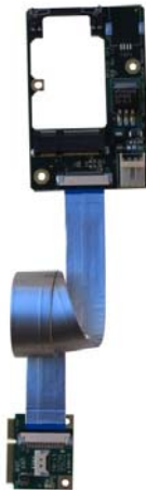
Figure 2: Flexible MiniPCI Express (half) Riser
