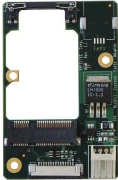
Figure 5: MiniPCI Express Adapter board
