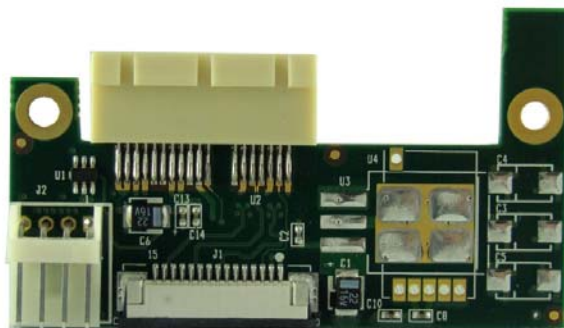
Figure 4: x1 PCI Express adapter board (powered from host card (3.3V only))
