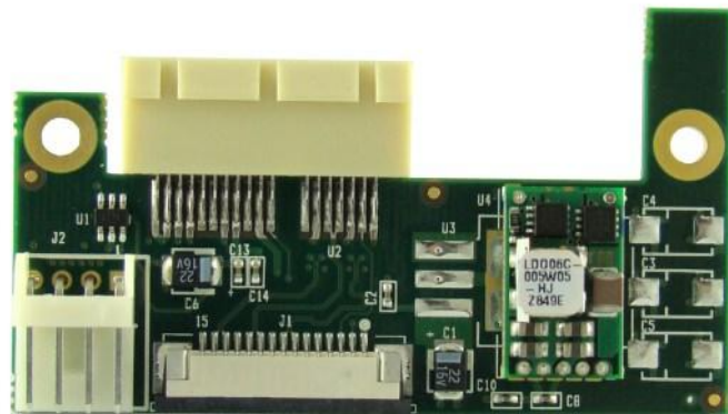
Figure 6: x1 PCI Express adapter board (powered from external 12V power supply)
